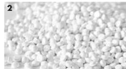
These flakes are heated to eliminate any impurities, then melted and transformed into dense **pellets**.
