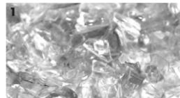
Instead of being burned, used drinking bottles are collected, sorted by colour and washed. After being stripped of their labels and caps, the bottles are crushed and cut into **PET flakes**.
